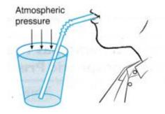
A siphon is a tube used to make liquid travel upwards from a container and then down to a container at a lower level unaided. For the water to go into the tube, air must be removed from the tube. Atmospheric pressure pushes water into the tube and then gravity causes it to flow down to the container at a lower level.
